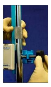
·Loosen the black knob on the pole clamp and secure it to the IV Pole
