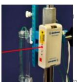
• Activate the laser by pressing and releasing red power button (Laser will stay on for 20-30 seconds, then turn off automatically)
